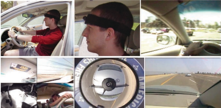
Fig. 9.1 Top: Head-band “3rd Eye” camera (left and middle) and view from it (right). Bottom: Example views from selected other cameras (composite on left, omniview in center, and rear view on left)
