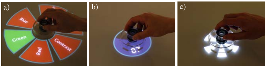
Fig. 7.9 SLAP Knob user interface. a) Selecting image property from menu. b) Setting continuous value. c) Relative navigation for frame stepping in videos
