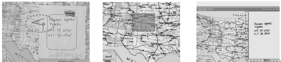
Fig. 6. Stitching a post-it note to a map. (left) Draw the stitching mark on paper. (middle) The resulting “anchor” region in the digital version. (right) Expanded “anchor” region for details. Figures are highlighted for clarity.
