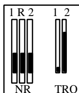
Figure 8. Number one engine low side failure. N_r indicates a decrease in power and TRQ indicates a significant split.
