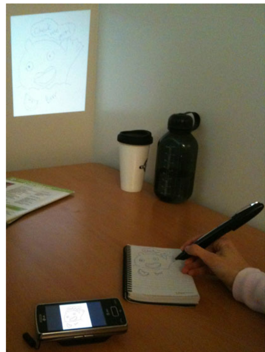
Fig. 2 Projecting while using UbiSketch. Phone screen and projected display show digitized version of paper sketch
